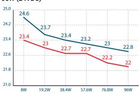
Output Voltage vs. Load
