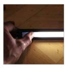
Wave your hand 1-4" from the sensor to turn on / off. Hold your hand in front to dim.
