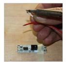
Strip your 18-22AWG stranded wire approximately 1/8". Tin the exposed wires with solder.
