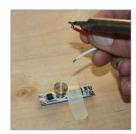
Strip your 18-22AWG stranded wire approximately 1/8". Tin the exposed wires with solder.
