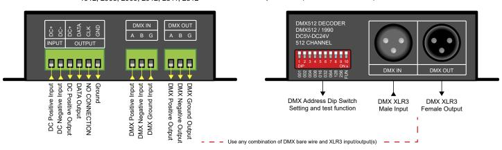
Digital IC type LED lights have a directional data input/output flow, you must follow this flow or you will damage the modules. Always input your data signal to the "DI" wires (DATE INPUT). Never wire from your DMX decoder to the "DO" wires (DATA OUTPUT). When cutting and connecting modules be sure to never reverse the flow of the modules. Arrows are printed on the modules to distinguish the directional flow, do not reverse this direction.
