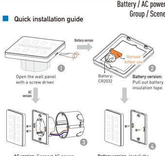
AC version: Connect AC power and install bottom part to socket with screw, then clip panel part to bottom part.
