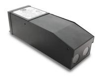
Magnitude's M200L24DC is the most compact LED driver on the market with a magnetic transformer core. It is equipped with 1 pushto-reset circuit breaker on the output, which protects both the load and driver. The driver is encased in a coated metal box that includes 2 knock-outs on the bottom to enable easy installation that complies with electrical code requirements.
