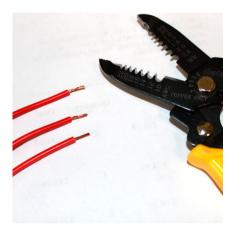
Start with your 16-22AWG DC stranded or AC solid wire pairs. Strip .25" off the ends of each wire.
