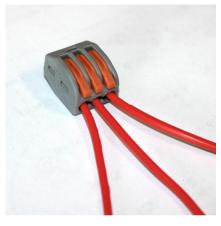
With the clamps in the up position insert your wires and then gently push the clamps down. Gently pull on the wires to be sure they are secure and then test for continuity.
