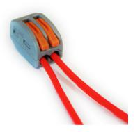
**3.)** With the clamps in the up position insert your wires and then gently push the clamps down. Gently pull on the wires to be sure they are secure and then test for continuity.
