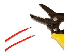
**1.)** Start with your 16-22AWG DC stranded or AC solid wire pairs. Strip .25" off the ends of each wire.
