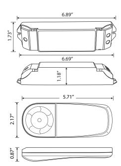
**PRODUCT NAME** Color Wheel RGB Sync Controller and Receiver Kit - 5-24VDC 6A/CH
