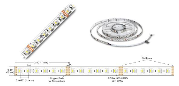
**PRODUCT NAME** Ribbon Star 50/50, High Density 4 in 1 RGBW LED Strip Light - ETL 24VDC - 19.5"(0.5m)
