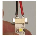
This is what a proper installation will look like, now test by connecting lead wires to a power source.
