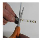
You can cut the ribbon on the line between 4 copper dots. Be sure to cut straight across.
