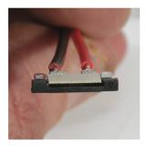
This is the top of the connector. You will place the Ribbon into this slot facing up.
