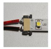
Insert Ribbon into connector, check the wire polarity (red wire to positive) copper dots should not be visible.
