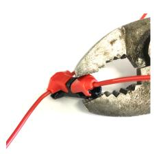
**2.)** Using a pair of pliers firmly snap the connector top down. The small red tabs on the bottom will click into place.
