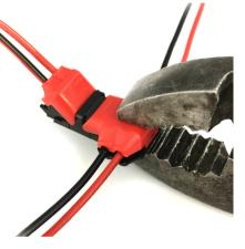
**2.)** Using a pair of pliers firmly snap the connector top down. The small red tabs on the bottom will click into place.
