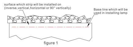
2. Fix the clip on the base line, and the distance depends on practical situation, figure 2, figure 3;
