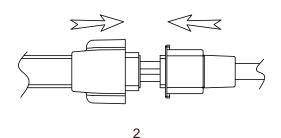
Push the external fastening buckle and front connector inward slowly until joint
