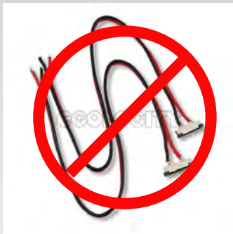
NO CONNECTORS (Strip light must be soldered)
